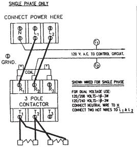
2 HEATING ELEMENTS - SINGLE PHASE ONLY DO NOT WIRE 2 ELEMENTS 3 PHASE NOTE: A 2 POLE CONTACTOR MAY BE USED ON MODELS HAVING A LOW WATTACE HEATER
