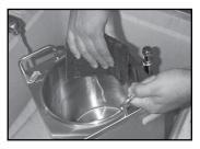
**NOTE** - Polish stainless steel surfaces with stainless steel polish after drying. This will prevent surface scratches and result in a cleaner appearance.
